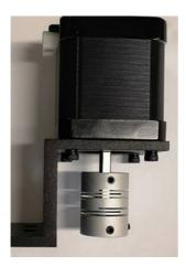
Note: Rotate the coupler slightly until one of the grub screws faces directly over the flat surface on Y Motor Shaft
