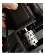
13. Hold up Y motor and pre-tighten the four screws which hold the motor on the frame.
