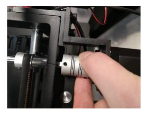
If motion is not smooth, it is not aligned. If not aligned adjust the position of the Y motor until the coupler can sl smoothly.
